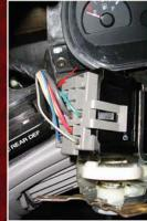
The black (negative) wire can be connected either to the ground (black) in this connector, or it can be grounded to a hole drilled in the chassis using a ring terminal and the enclosed nut and bolt.
